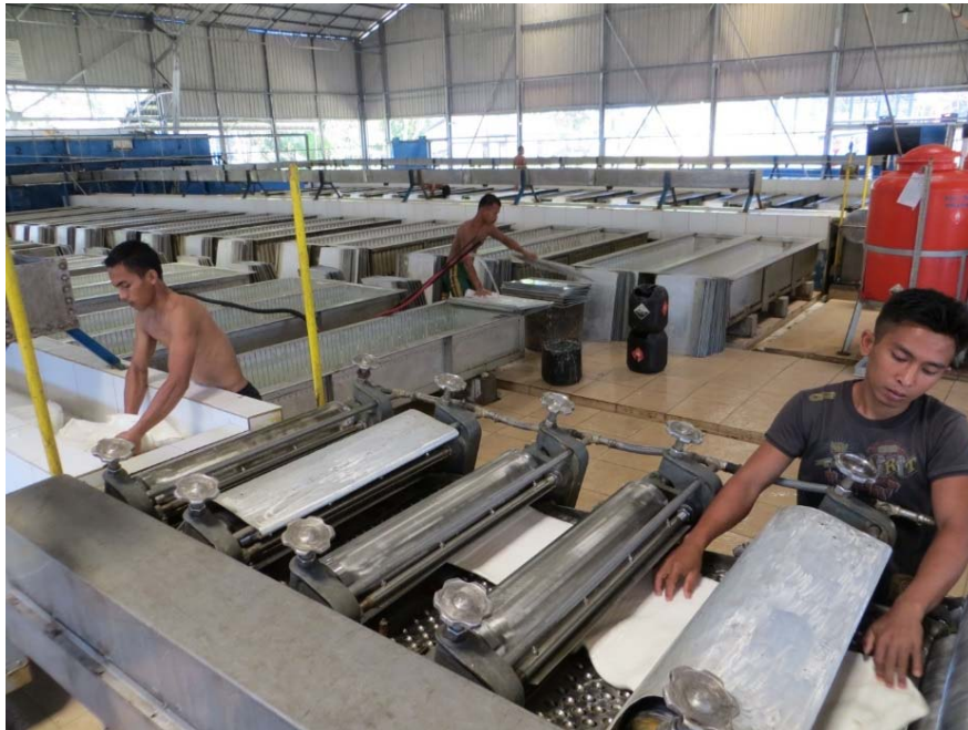
Coagulated latex slabs are then milled using multi-roll crepes.
