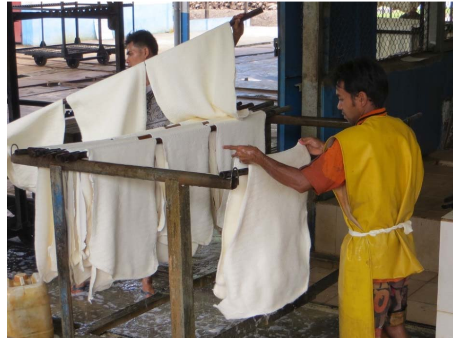
Thin sheets at 3mm are produced.
